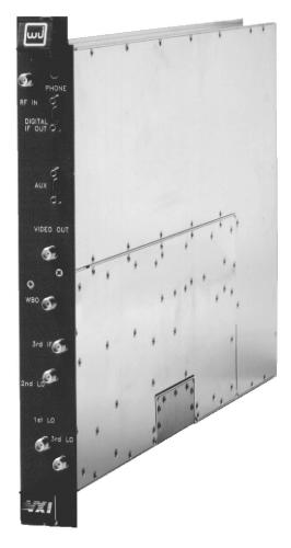
The WJ-8621 is a general-purpose VHF/UHF receiver covering a 20 to 2700 MHz frequency range. WJ packages the unit in a single-slot C-size VMEbus extensions for Instrumentation (VXI) module. The WJ-8621 is ideal for applications requiring broad-frequency coverage in a highly integrated package. Combining receiver control directly onto a standard instrumentation and computing bus adds significant system capabilities, yet reduces the complexity of system integration.
